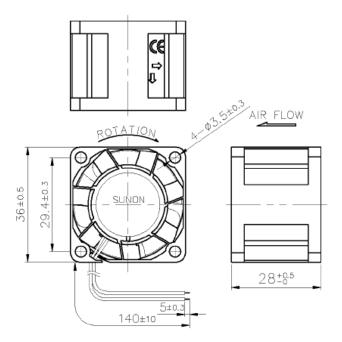
NOTE: 1. LEAD WIRE: UL1571 #28AWG +: RED WIRE -: BLACK WIRE 2. FRAME TYPE: RIB
