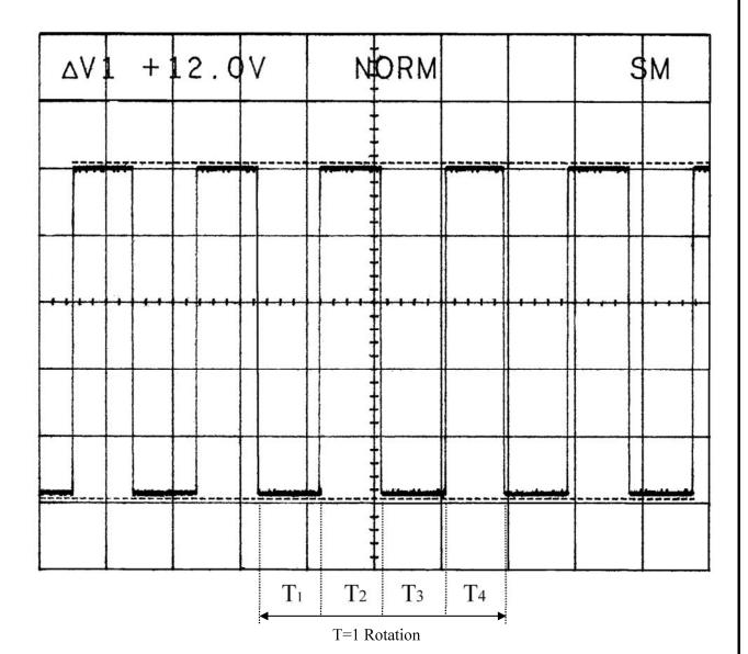
T=T1+T2+T3+T4 =(1 Rotation) T1=T2=T3=T4= $\frac{60}{4 \times \text{rpm}}$
