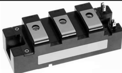
dual switch (half-bridge)
